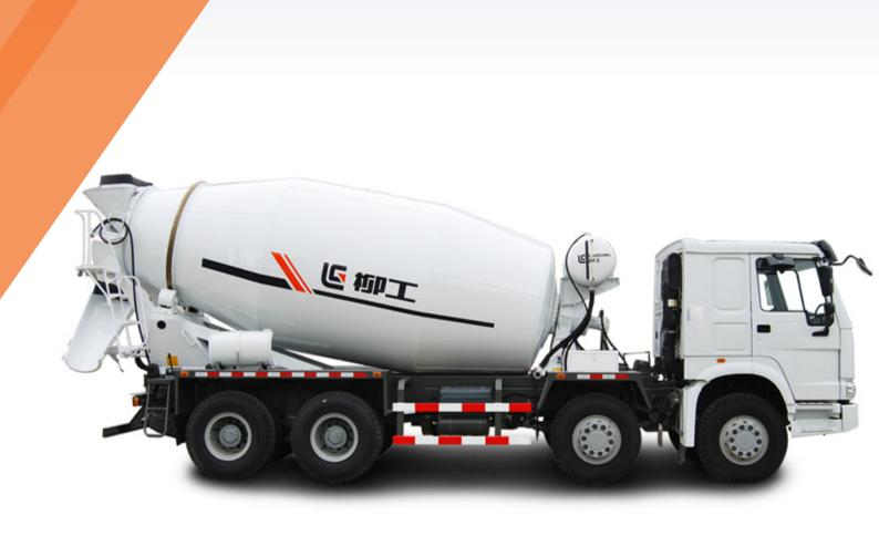
Drum Geometrical Volume Drum Agitating Capacity Concrete Charge Speed Concrete Discharge Speed Drum Remnant Ratio Drum Inclined Angle Water Reservoir Capacity Water Supply Type 19.2 m<sup>3</sup> 12 m<sup>3</sup> ≥ 3 m<sup>3</sup>/min ≥ 2.7 m<sup>3</sup>/min < 0.5% 11° 450 L Pneumatic Pressure
