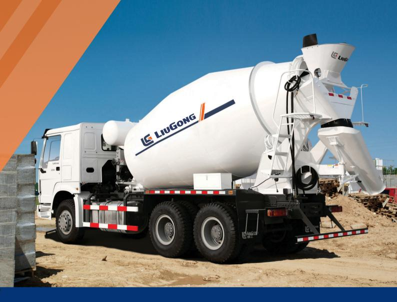
Drum Geometrical Volume Drum Agitating Capacity Concrete Charge Speed Concrete Discharge Speed Drum Remnant Ratio Drum Inclined Angle Water Reservoir Capacity Water Supply Type 17.2 m<sup>3</sup> 10 m<sup>3</sup> ≥ 3 m<sup>3</sup>/min ≥ 2.7 m<sup>3</sup>/min < 0.5% 12.5° 450 L Pneumatic Pressure
