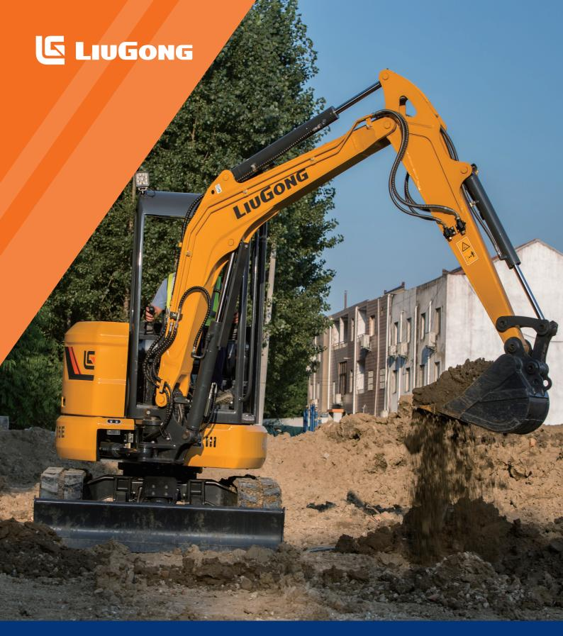
EngineYanmar 3TNV88-BPLYRated Power22.2 kW (29.8 hp / 30.2 ps) @ 2,400 rpmNet Power21.2 kW (28.4 hp / 28.8 ps) @ 2,400 rpmMaximum Dig Depth3,085 mmStandard Bucket Capacity0.11 m³Operating Weight (with Cab)3,980 kgOperating Weight (with Canopy)3,860 kg
