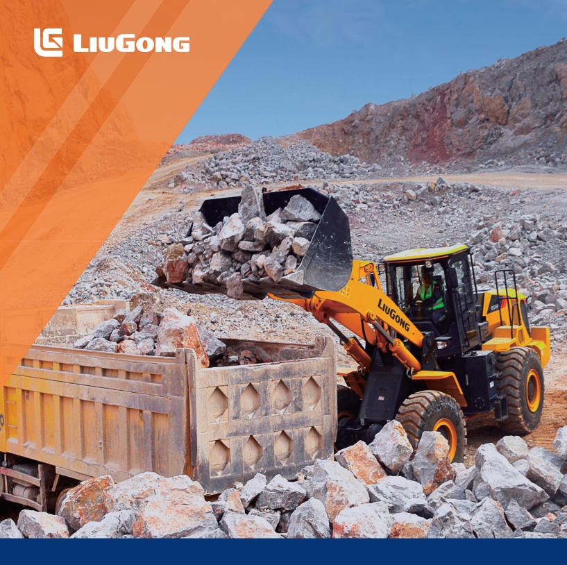
Engine Cummins 6LTAA9.3 Gross Power 162 kW (217 hp / 220 ps) @ 2,200 rpm Net Power 154 kW (207 hp / 209 ps) @ 2,200 rpm Operating Weight 17,250 kg Standard Bucket Size 3.5 m³ Standard Breakout Force 172 kN Standard Dump Clearance 3,013 mm
