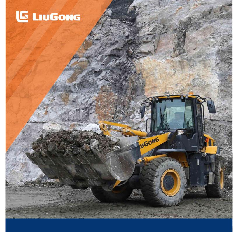
EngineWeichai WP6G175E201Rated Power129 kW (173 hp / 175 ps) @ 2,000 rpmNet Power119 kW (160 hp / 162 ps) @ 2,000 rpmOperating Weight13,075 kgStandard Bucket Size2.3 m³Standard Breakout Force124 kNStandard Dump Clearance2,889 mm
