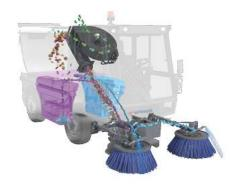
The 2-broom system with independently controlled circular brushes guarantees absolute mobility in every sweeping situation. Two stable broom arms with integrated buffers allow sweeping widths of up to 2,900 mm.
