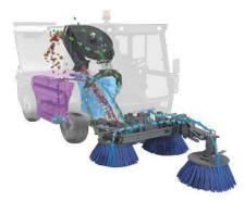
The 3-broom system with freely movable front brush arm offers a sweeping width of up to 2,600 mm. Left-right alignment of the front broom is just as possible as sweeping on two levels or heavy weed broom use.
