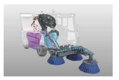
adding water into the hopper, up to 250 litres, the operating range can be increased by up to 50%. The collected swept material is both moistened and compacted. The electric fresh water pump supplies the spray nozzles on the circular brooms. The water quantity for the brooms can be conveniently controlled from the cab.
