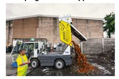
The hopper, which has a system volume of 2m³, enables maximum sweeping capacity and a large radius of action. The hopper is made of corrosion and seawater resistant aluminium. A large dumping height of 1400mm enables emptying into all common dirt containers. The suction pipe in the hopper is optionally available in wear-resistant stainless steel.
