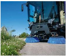
A flexible sweeping system helps ensure thorough cleaning in any situation. The towed disc brush system, mounted in front of the front axle, achieves a sweeping width of 2,200 mm.
