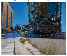
With the optional third brush, the span swept can be as wide as 3,550 mm. This allows a larger area to be covered as well as sweeping on two levels.
