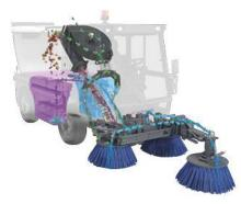
The 3-broom system with freely movable front brush arm offers a sweeping width of up to 2,600 mm. Left-right alignment of the front broom is just as possible as sweeping on two levels or heavy weed broom use.
