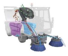
The 2-broom system with independently controlled circular brushes guarantees absolute mobility in every sweeping situation. Two stable broom arms with integrated buffers allow sweeping widths of up to 2,900 mm.
