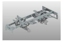
payload in its class - up to 6,600 kg thanks to robust suspension, high axle loads and twin tyres on the rear axle. A large steering angle of 68°, combined with the short wheelbase of 1,850 mm, allows optimum manoeuvrability and an extremely tight turning circle.
