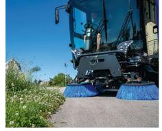
A flexible sweeping system helps ensure thorough cleaning in any situation. The towed disc brush system, mounted in front of the front axle, achieves a sweeping width of 2,200 mm.
