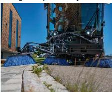
With the optional third brush, the span swept can be as wide as 3,550 mm. This allows a larger area to be covered as well as sweeping on two levels.
