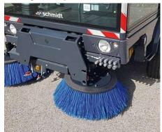
A flexible sweeping system guarantees a clean result in every situation. The pulled disc brush system mounted in front of the front axle has a sweeping width of 2,200 mm.
