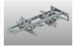
highest payload in its class - up to 6,600 kg thanks to robust suspension, high axle loads and twin tyres on the rear axle. A large steering angle of 68°, combined with the short wheelbase of 1,850mm, allows optimum manoeuvrability and an extremely tight turning circle.
